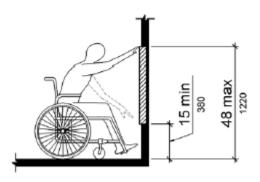
• Where a high forward reach is over an obstruction, the clear floor space shall extend beneath the element for a distance not less than the required reach depth over the obstruction. The high forward reach shall be 48 inches (1220 mm) maximum where the reach depth is 20 inches (510 mm) maximum. Where the reach depth exceeds 20 inches (510 mm), the high forward reach shall be 44 inches (1120 mm) maximum and the reach depth shall be 25 inches (635 mm) maximum.
